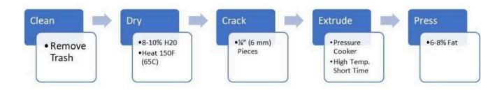
By quickly cooking seeds in about 20 seconds (compared to 20 minutes in traditional cookers), extrusion:
